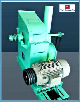
Hammer mill comprises of a heavy duty mild steel fabricated body (alternatively stainless steel construction can be provided in hammer mill wherever necessary). The grinding chamber of hammer mill is lined with serrated wear plates, which protects the body from wear and tear. A dynamically balanced rotor in hammer mill with a set of swing hammers accelerates the grinding process. The screen classifier forms the lower half of the grinding chamber of hammer mill.
